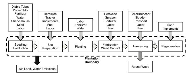
Figure 2. Schematic of the life cycle inventory serving as the basis for calculating the global climate change impacts of anthropogenic activities, adapted from Turn et al. [38].
